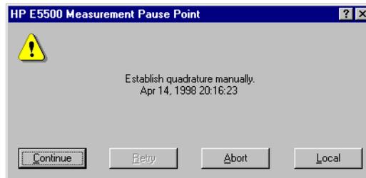
2. First establish quadrature by adjusting the phase shifter until the meter indicates 0 volts, then press Continue.
